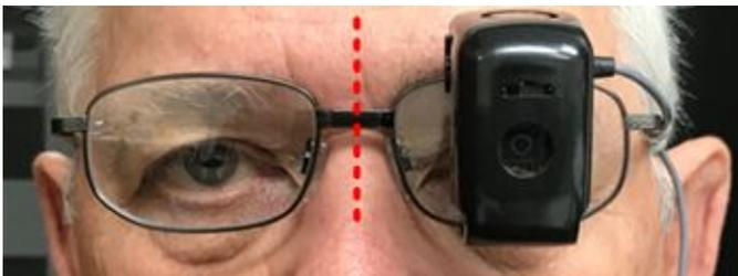
Looking down on the patient's head, confirm the ocular is centered horizontally onto the pupil. If not, offset nose pieces slightly to compensate for that misalignment.
